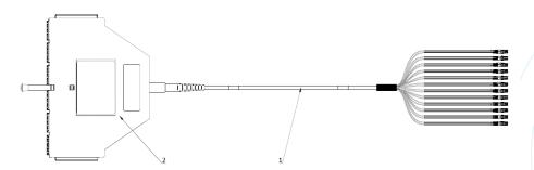
√ NGX LC Module – Pre-terminated 24FO to 12 LC Duplex tailored Staggered Fanout
