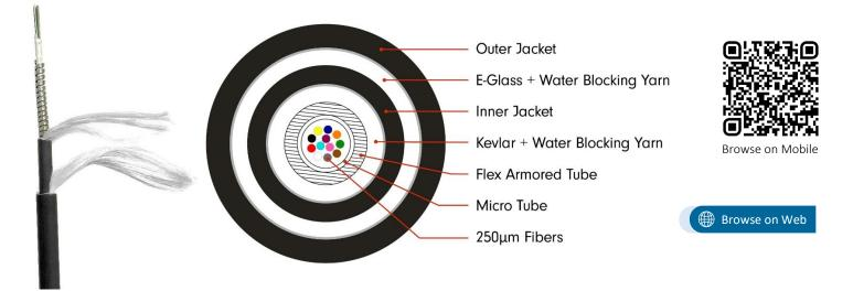
NEXCONEC<sup>®</sup> Indoor & Outdoor Microcore Flex Armored cable contains 12 fibers of 250µm fibers in a micro tube, which is accommodated in the helical flex armored tube, then with E-glass, Kevlar and water blocking yarn added in the cable to make ideal use in the indoor/outdoor environment where anti-rodent is needed.
