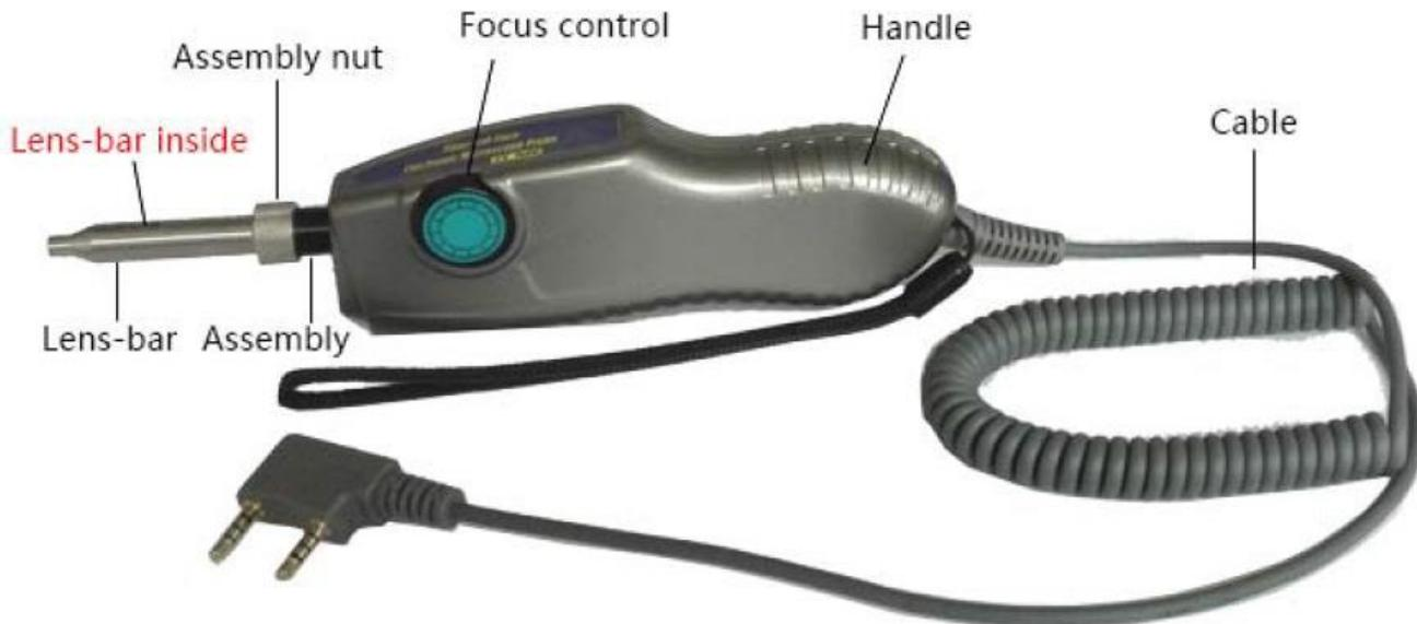
1. **Handle:** also named as probe, all the optical routines are concentrated inside the handle, responsible for the fiber imaging.
