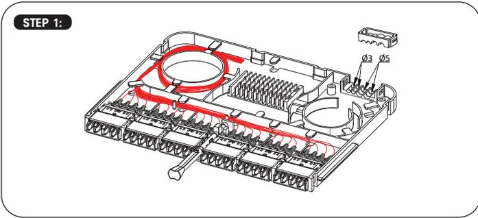
Remove the plastic cable clamp and choose the cable/tube slot from one of the 4 slots as per installation requirements. (Picture shown above)
