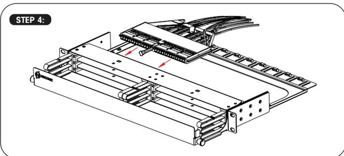
Insert patching module from rear side of the panel & keep enough margin of patchcords in the rear side to make sure easy movement of the module.
