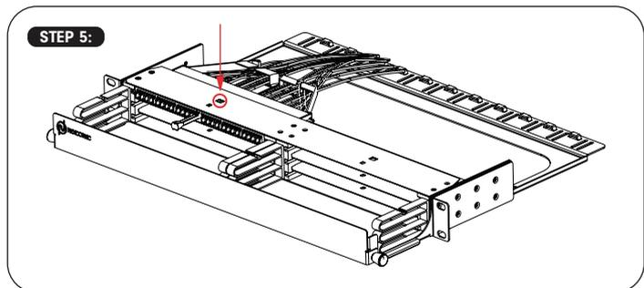
Rotate the push/pull tab of the module into lock position to restrict its movement.
