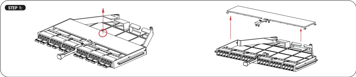
Use two fingers to pick the middle area of lid (as shown above in pic-1) and lift up to easy remove the lid from module to access patching adapters.
