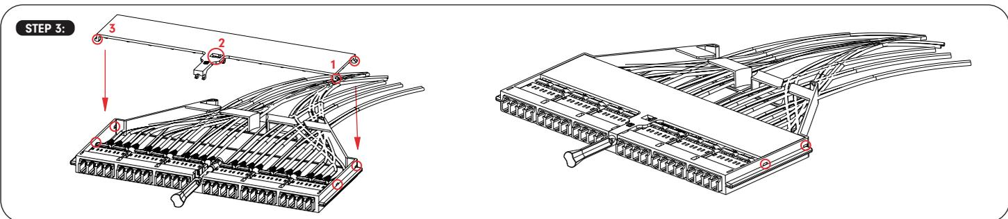
Insert back the lid by matching lid flange (1) with module holes, then match middle part (2) and hold middle area with a thumb and then match lid flange (3) with module holes to make easy and perfect fit.
