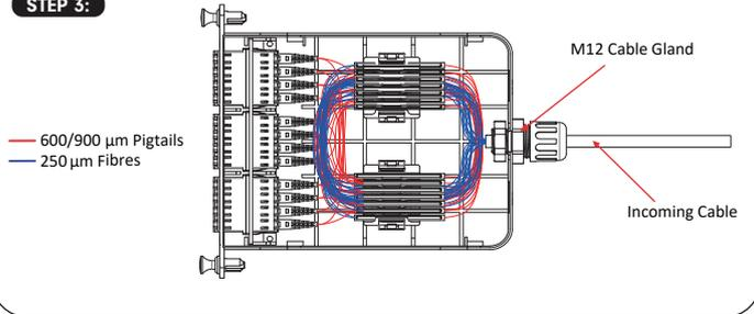
Above picture is the cassette fully spliced with 2 sets pigtails.
