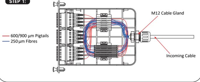
Splice the 1<sup>st</sup> set 12 rainbow pigtails as above picture shown (Please cut the 600/900µm pigtails according to the real installation).
