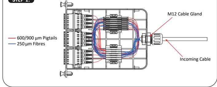
Splice the 2<sup>nd</sup> set 12 rainbow pigtails as above picture shown (Please cut the 600/900µm pigtails according to the real installation).
