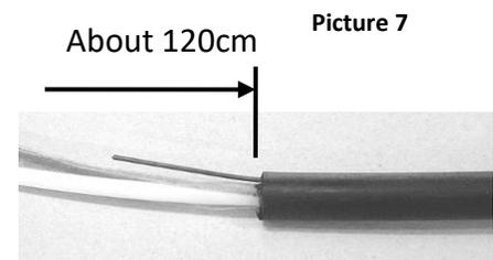
2.2.2.4 Cut off the extra reinforced core about 5cm from the removing point on the sheath.
