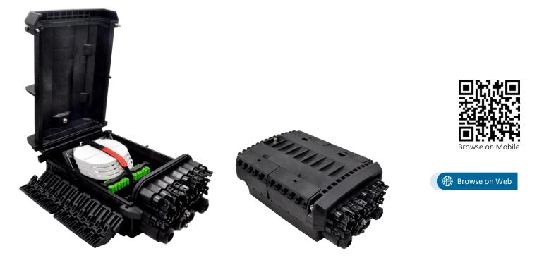
OC-DO03B/C is used as a termination point for the feeder cable to connect with drop cable in FTTH network system. It is designed to seal without screws. The compact size and flip-over cover bring easy operation as well as multi-purposes applications. It could be installed in aerial, wall, pole and pipe line mounted mode.
