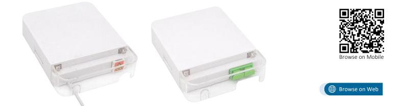
The compact termination box supplied by NEXCONEC<sup>®</sup> is designed for use in residential and business applications for the termination of up to four fibers. This wall box enables the installation of either a single Sirocco Blown Tube cable using up to a 2 fiber blown unit or two 2 fiber ruggedized cables to be spliced to 2 SC pigtails (PC or APC), which connect to adapters at the base of the unit.
