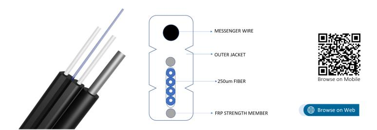
NEXCONEC® FTTH Drop Cable is made of 1 to 4, 250μm individually colored optical fibers with fiber reinforced strength members, steel wire which also acts as messenger wire and UV resistant Low Smoke Zero Halogen (LSZH) or PE jacket. The steel wire provides additional strength suitable for aerial applications.
