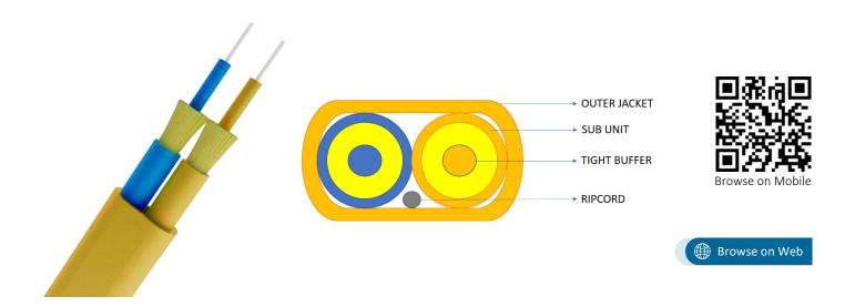
NEXCONEC® Flat Duplex Fiber Optic Patch Cable is manufactured with two simplex units held together with an overall Low Smoke Zero Halogen (LSZH) or PVC jacket. Ideal for use in office LAN connections, Patch Cords, and internal point-to-point links where frequent handling is likely.
