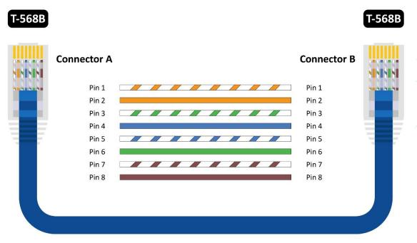
STRAIGHT-THROUGH WIRING (Nexconec Standard)
